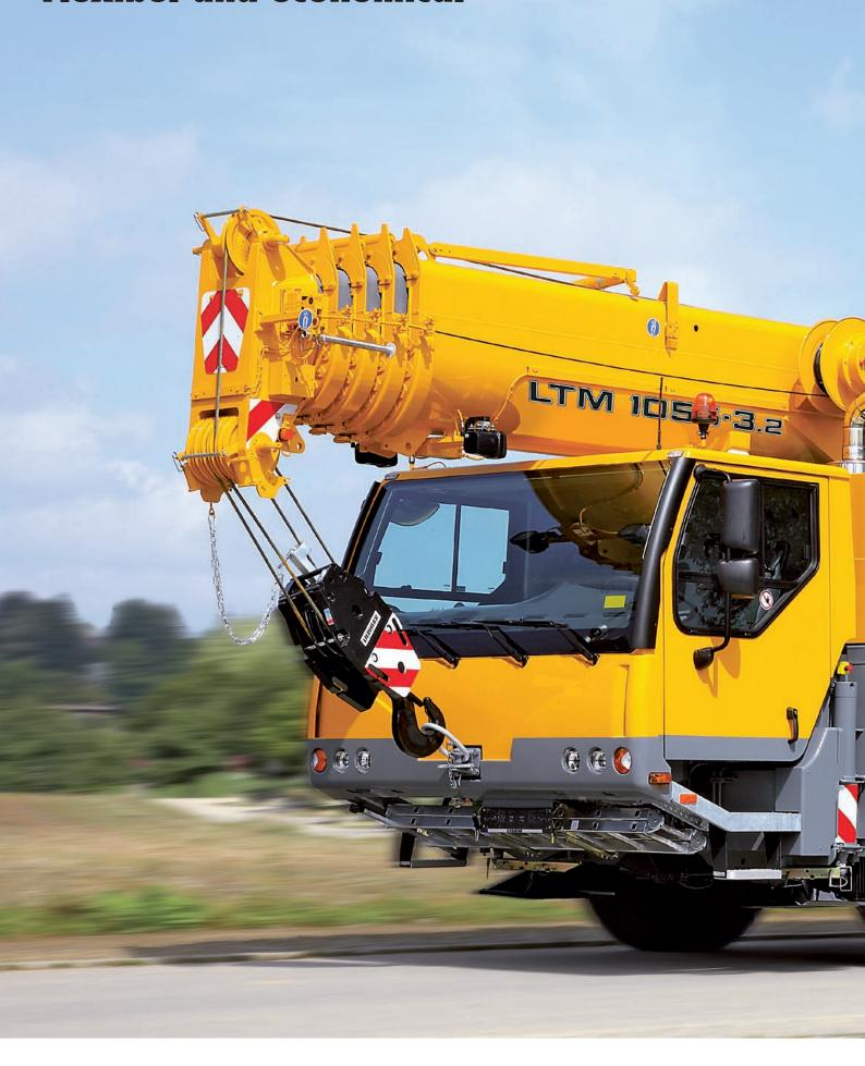
A long telescopic boom, high capacities, an extraordinary mobility as well as a comprehensive comfort and safety configuration distinguish the mobile crane LTM 1055-3.2 from Liebherr. The 55-ton crane offers state of the art technology for more convenience for the practical operation.
